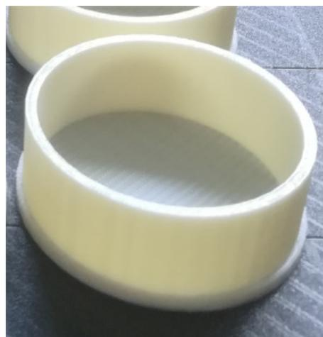
**Fig. 1.** Mould for suction controlled oedometer test [8].
