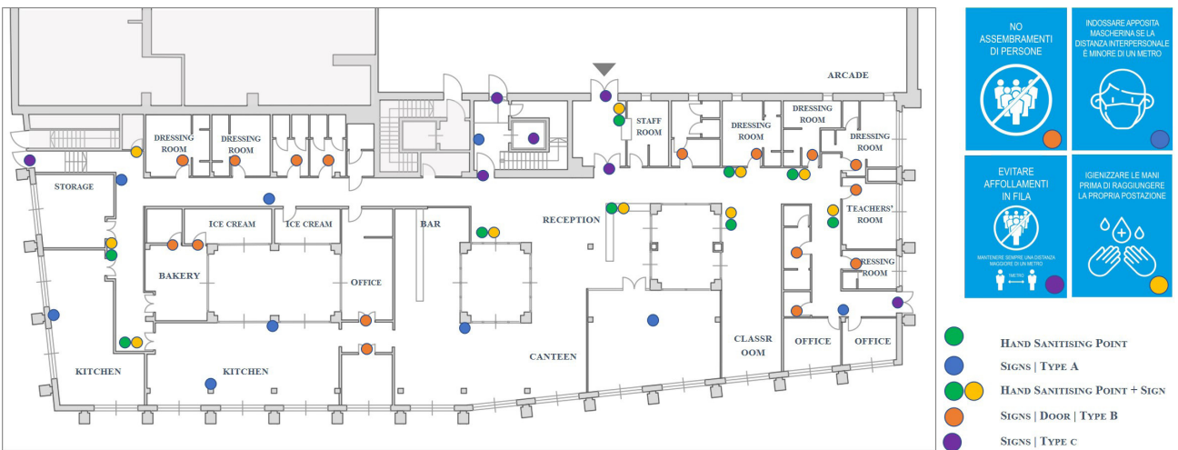
Figure 13. Ground floor plan with indication of the positions of some categories of communication signs.
