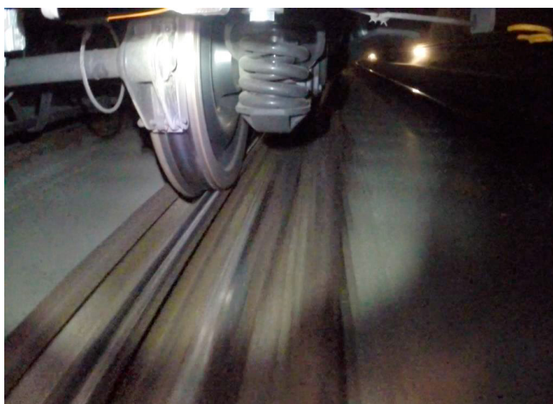
Fig. 11. Detail of one vehicle wheel while running on the switch located at km 37 of the Gotthard Base tunnel.
