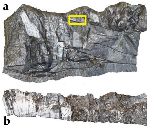
Figure 9. Point cloud representing (a) the entire quarry (in yellow the location of bench in the quarry); (b) the studied bench.
