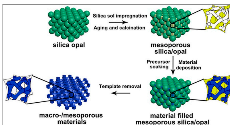
Figure 1. Schematic representation of 3D macro/mesoporous materials preparation reproduced with permission from [34], Chemistry of Materials, 2018.
