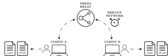
Figure 1: Testbed setup and RTC communication schema.
