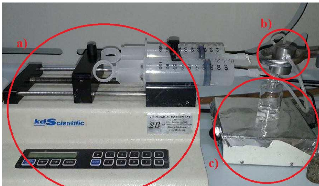
Figure 3.1. Nanoparticle production set up. The main elements highlighted are a) the syringe pump, b) the CIJM mixer and c) the collecting vial with quenching water and magnetic stirrer.
