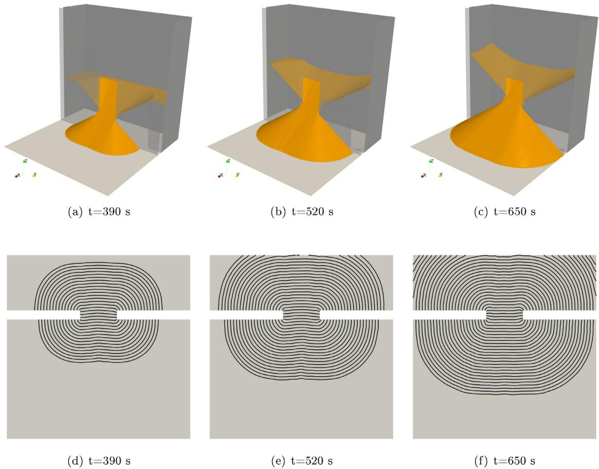
**Fig. 6.** Profiles of sand poured in the space behind the door and exiting from it at later times. The profile shown in (f) is almost stationary. All the sand poured between the walls falls off the open boundaries to the right and to the left. The sliding is achieved using the DPSM with a Coulomb closure. The bottom row reports the contour plots of the 3D configurations plotted in the top row.
