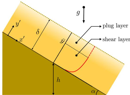
**Fig. 1.** Velocity profile within a layer of moving sand behaving like a viscoplastic fluid in the vertical section containing the direction of steepest descent. The layer has thickness  $\delta$  and  $\bar{y}$  distinguishes the shear layer for  $y' < \bar{y}$  (full curve) from the plug layer for  $y' > \bar{y}$  (dashed curve).
