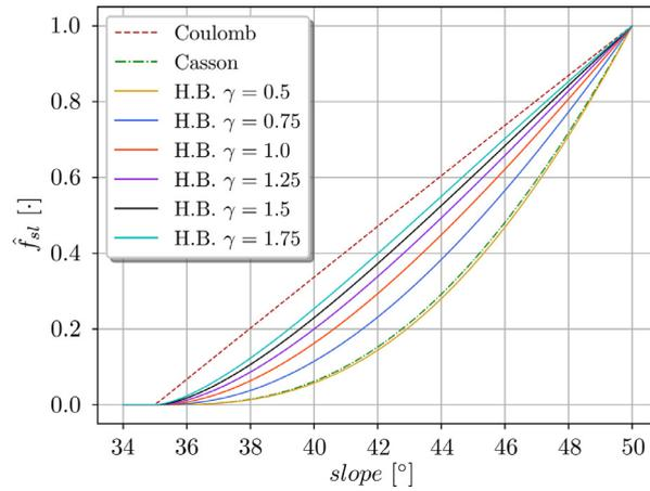
**Fig. 2.** Sliding term  $\hat{f}_{sl}^f$  normalized with respect to the value achieved for a slope of  $50^\circ$  and a repose angle of  $\alpha_{cr} = 35^\circ$  for different DPSM closure assumptions. We recall that Bingham fluids correspond to a Herschel-Bulkley model with  $\gamma = 1$ .
