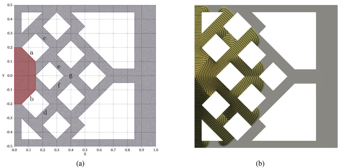
**Fig. 7.** (a) Domain of integration and numerical grid. The sand is poured in the shaded region in the grid. (b) Contour plot of the solution of the DPSM with Coulomb closure at  $t = 840$  s. Corners in the contour plots correspond to slope discontinuities of the sand profile.
