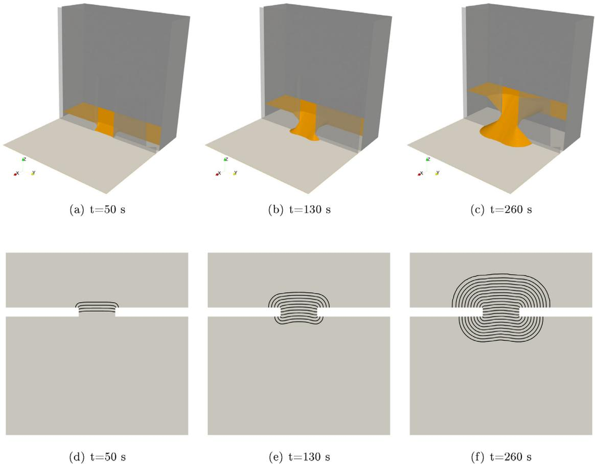
**Fig. 5.** Profiles of sand poured in the space beyond the door and exiting from it at early times. The sliding is achieved using the DPSSM with a Coulomb closure. The bottom row reports the contour plots of the 3D configurations plotted in the top row.
