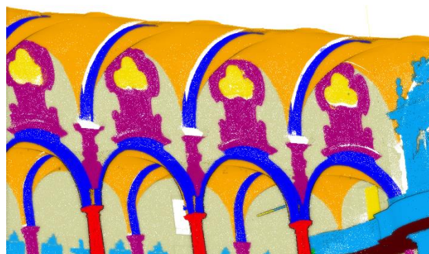
Figure 6. Examples of arches (blue) at a different height from the vaults (orange).
