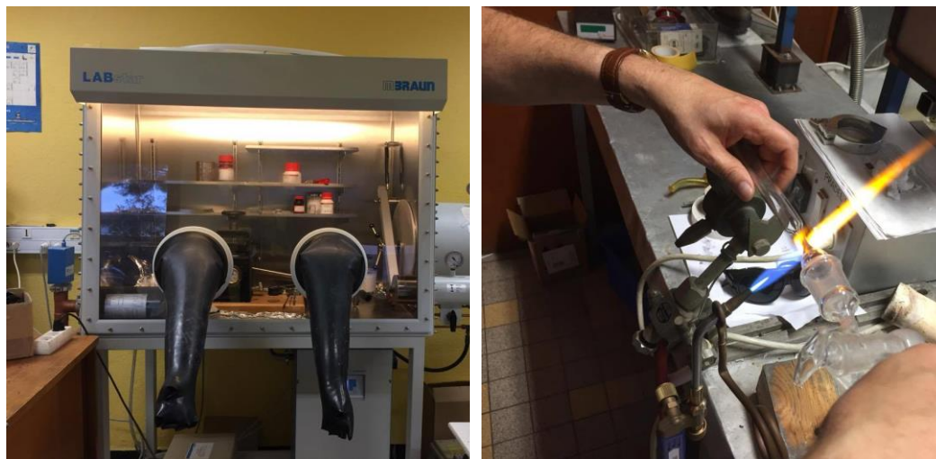
Figure 2.2 – Argon glovebox and a flame sealed tube.
