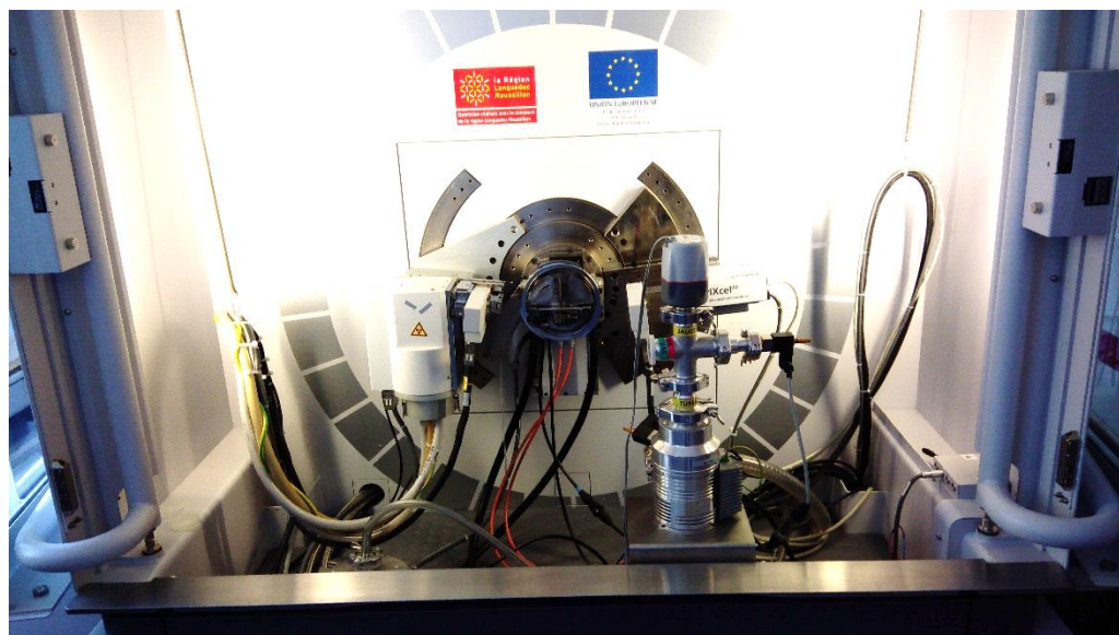
Figure 2.4 – Emphyrean PANalytical diffractometer for in-situ XRD experiments
