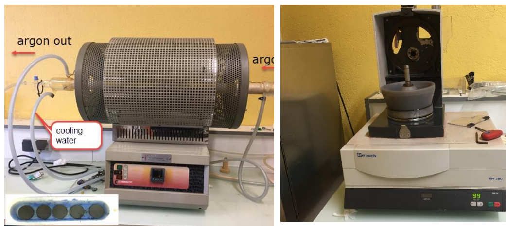
Figure 2.1 – The Ar-flow furnace setup for LaSrCoO 4 synthesis and mortar pestle machine.
