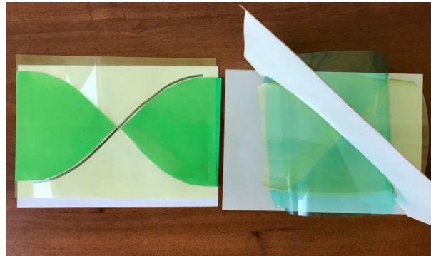
Fig.3. Flattened acetate sheets with evidenced sine function and cylinders intersecting in a plane. Photo credits by Maria Luisa Spreafico.
