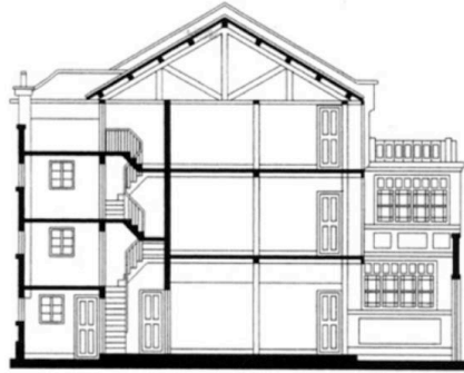
Figure 38 Late Shikumen section (Adapted from Zhao 2010)
