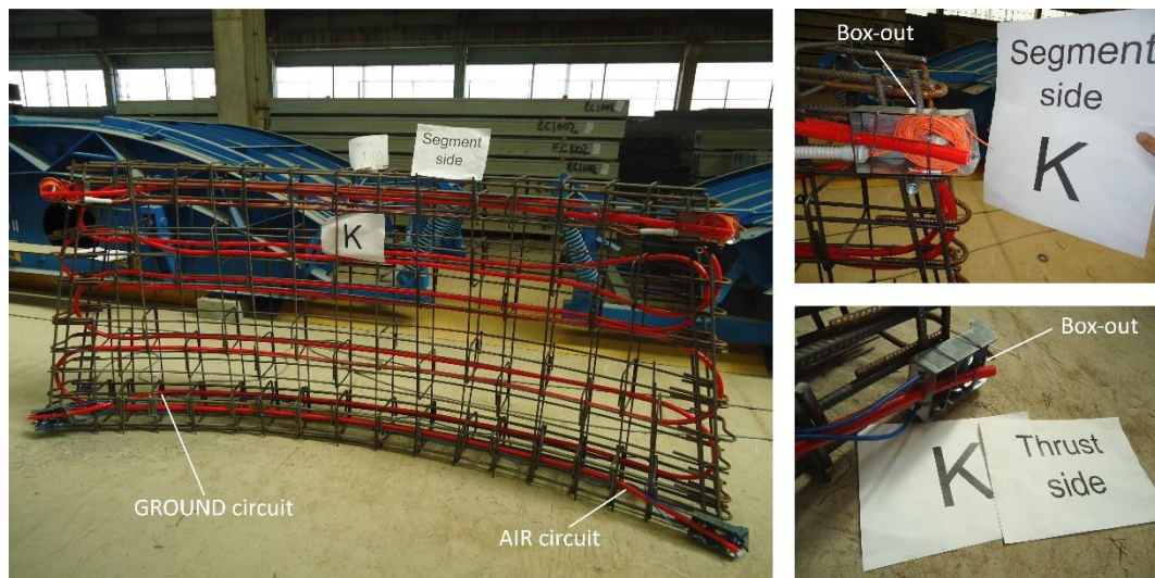
Figure 4.6: Example of steel cage equipped with pipes before casting (segment 1, ring 180) with detail of box-outs.
