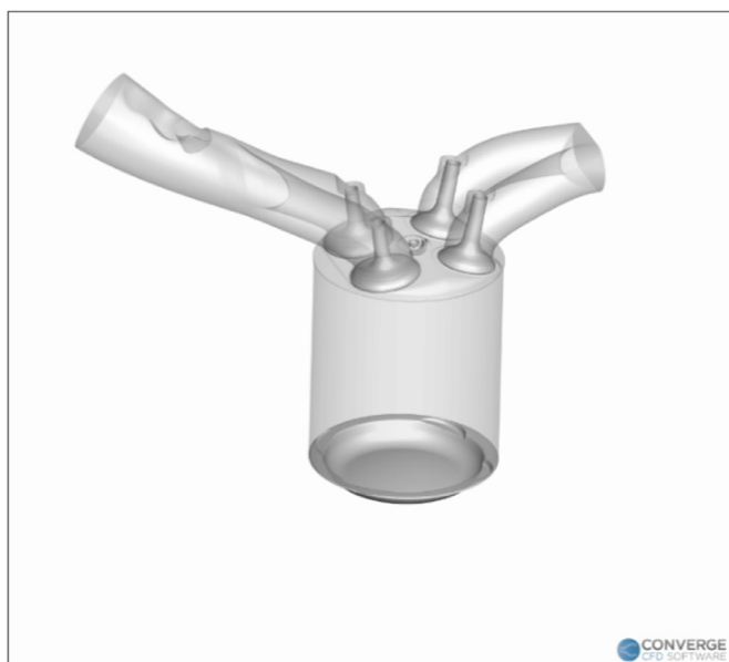
Fig. 1. CAD model of the engine combustion chamber, including intake and exhaust ports, valves and spark plug.
