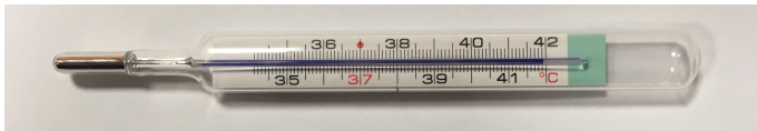
Fig. 6. A gallium thermometer, which replaced the glass mercury thermometers. The gallium bar read about 41.9 °C and has a silvering color.
