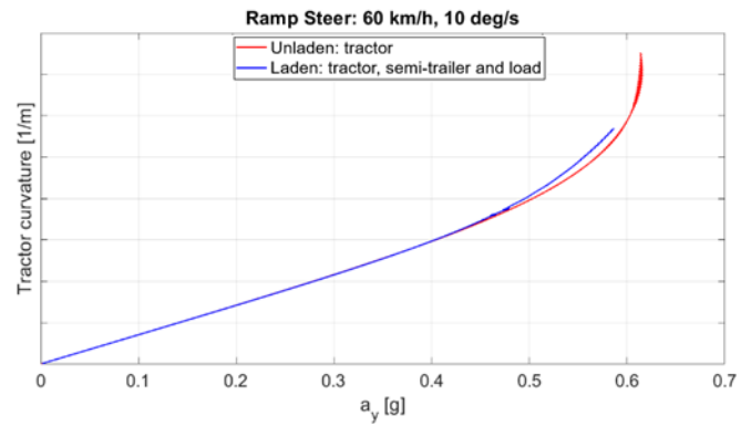
Figure 9. Ramp steer: Tractor curvature
