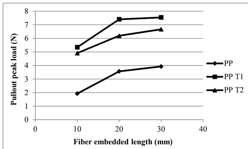
FIGURE 8. Maximum pullout load vs. embedment length
