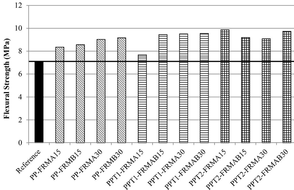
**FIGURE 9.** Comparison of fiber reinforced mortars flexural strengths
