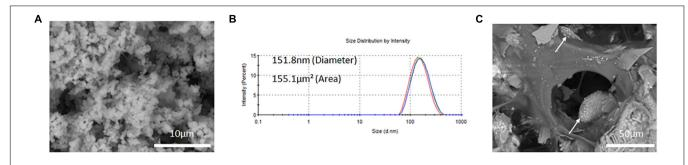
FIGURE 3 | (A) SEM image of free PLGA-DOXO NPs. Scale bar represents 10 μm. (B) Zetasizer DLS readings of PLGA-DOXO NPs suspended in DI water. (C) SEM image of PLGA-DOXO NPs loaded bone cement (40/60 composition) (visible as white spheres). Scale bar represents 50 μm.
