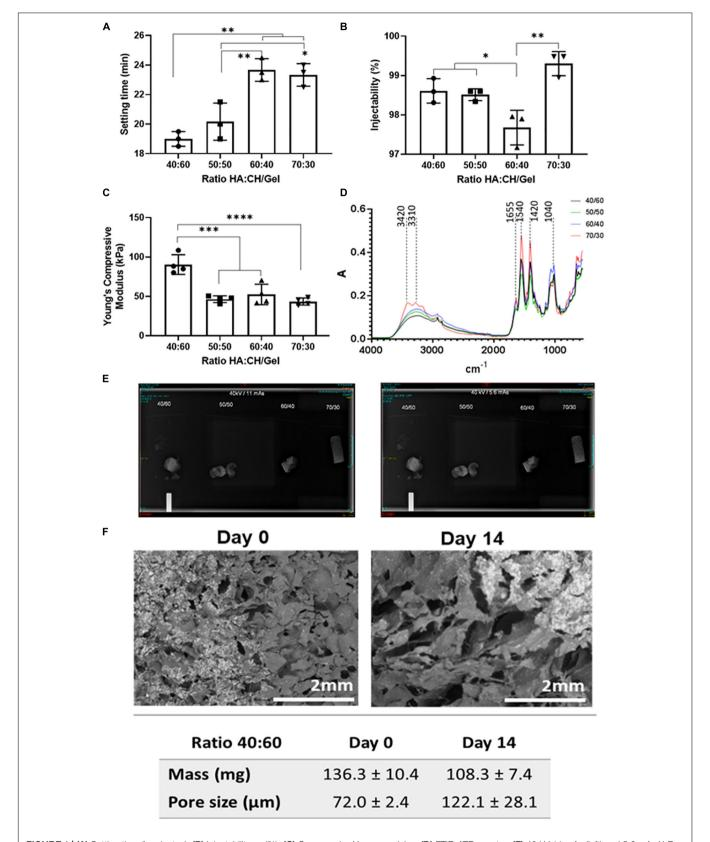
**FIGURE 1 | (A)** Setting time (in minutes), **(B)** Injectability as (%), **(C)** Compressive Young modulus, **(D)** FTIR-ATR spectra, **(E)** 40 kV 11 mAs (left) and 5.6 mAs X-Ray (right) Images visible for bone cements at different ratios of hydroxyapatite and Chitosan/Gelatin 40/60, 50/50, 60/40, and 70/30. **(F)** SEM micrographs of bone cements (40/60) after 14 days incubation in PBS at 37°C. Statistics:  $^*p < 0.05$ ,  $^*p < 0.007$ ,  $^*p < 0.0007$ ,  $^*p < 0.0001$ .
