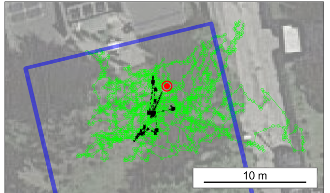
Fig. 3. Effects of the 3-layer low-pass GPS filter on dataset A.
