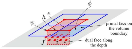
Fig. 2. Dual discretization of the conductive domain by considering the depth coordinate. Blue lines: primal grid. Red lines: dual grid.
