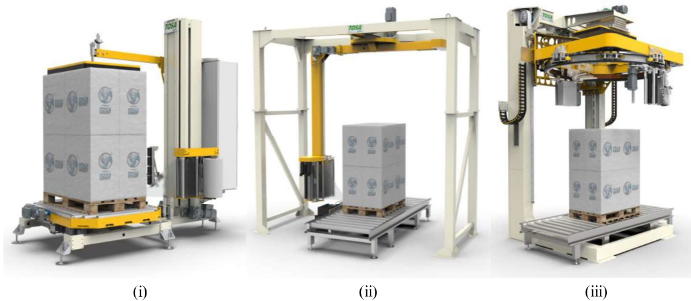
Figure 1 – Illustration of the three main categories of wrapping machines: (i) turn table, (ii) rotating arm and (iii) rotating ring.
