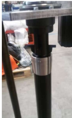
Figure 6 – Workstation no. 22: spindle group on pre-stretch frame plate assembly.
