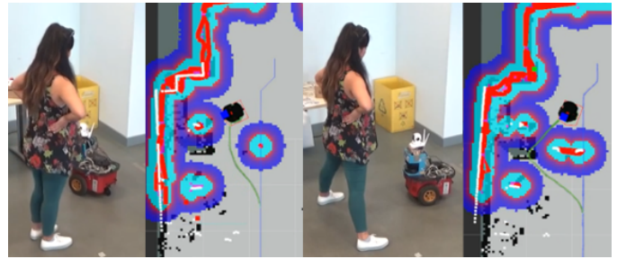
Fig. 1. The Sen3Bot human obstacle avoidance behaviour.
