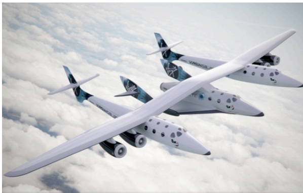
Figure 2: SpaceShip with its Carrier WhiteKnight, take off configuration [Credits: Virgin Galactic]
