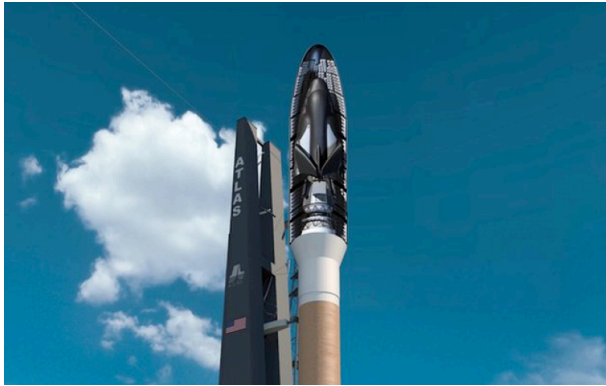
Figure 4: Sierra Nevada Dream Chaser in launch configuration
