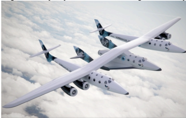
Figure 2 Shows the WhiteKnight2 and SpaceShip2 captive configuration at takeoff and flight to release altitude.
