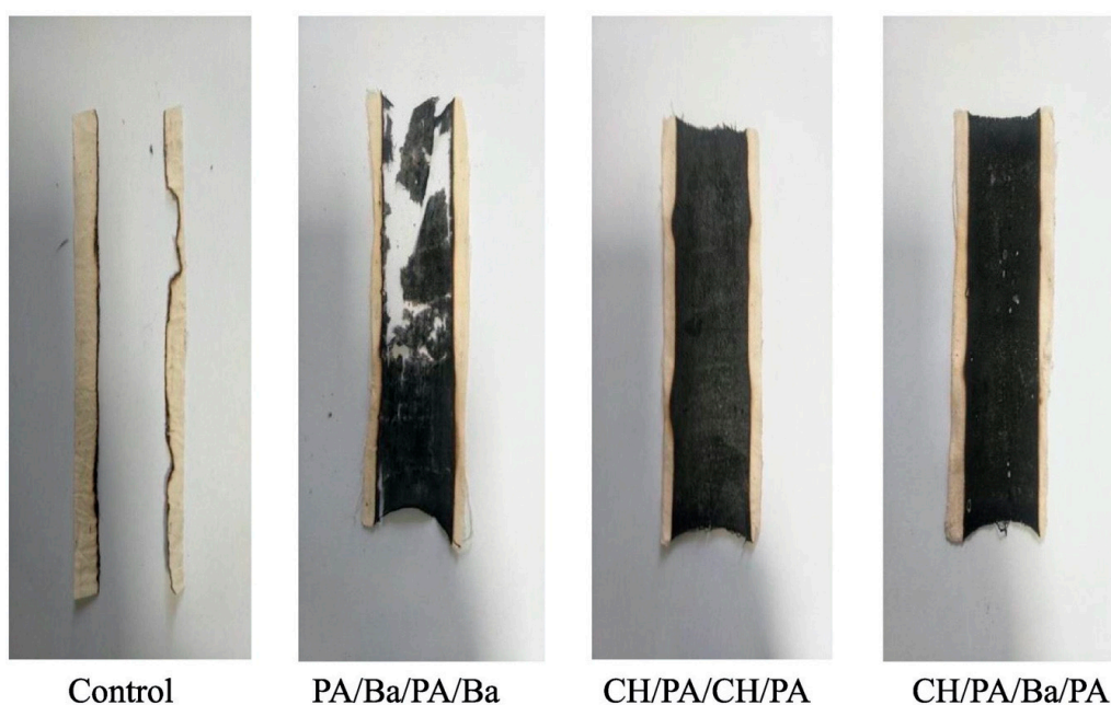
Figure 12. Residues at the end of the flame spread tests performed in a horizontal configuration. PA/Ba/PA/Ba: quad-layer made of phytic acid/Ba 2+ /phytic acid/Ba 2+ ; CH/PA/CH/PA: quad-layer made of chitosan/phytic acid/chitosan/phytic acid; CH/PA/Ba/PA: quad-layer made of chitosan/phytic acid/Ba 2+ /phytic acid. Reprinted with permission from [42]. Copyright 2019, Elsevier.
