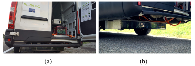
Fig. 4: Receiver structure mounted under the vehicle. Rear view (a), with the PE in the red box inside the vehicle. Detailed view (b).
