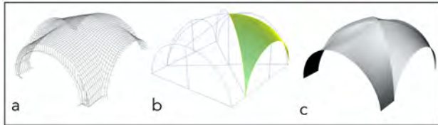
Figure 6. NURBS modelling strategy: from planar sections (a) to simplified wired profile on which surfaces have been modelled (b) to final model (c).
