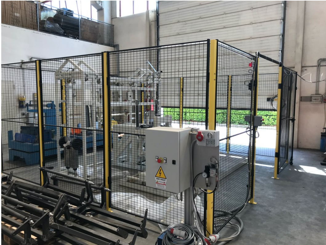
Figure 114: Safety grating and control panel of the test bench
