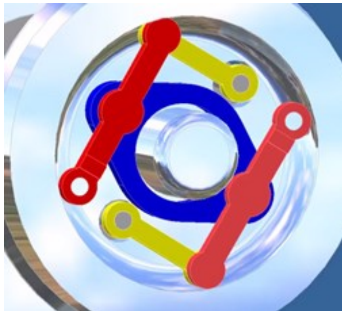
Figure 113: Detail of the quill drive mechanism
