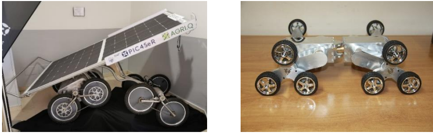
Fig. 1. Agri.Q and Epi.Q, UGVs composed of two differential driven modules linked together.
