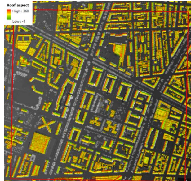
Figure 4. Roof aspect analysis (orientation, degree)
