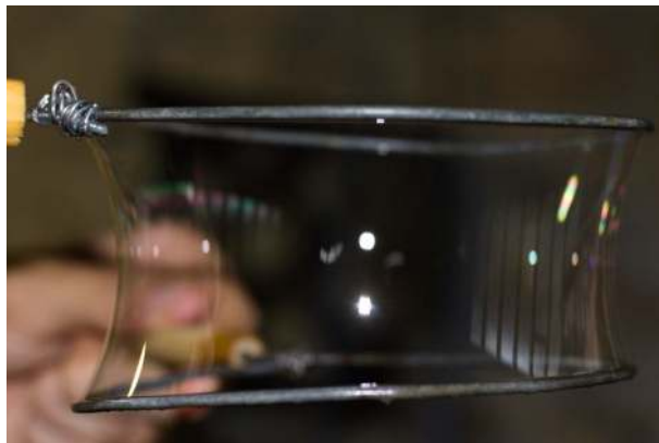
Figure 2: A catenoid as a soap film that spans two coaxial rings.
