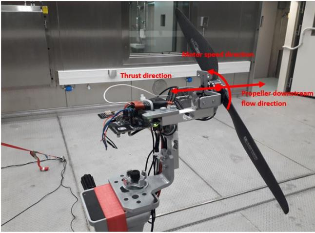
Fig. 2: Propeller mounting on the RCBenchmark thrust stand.
