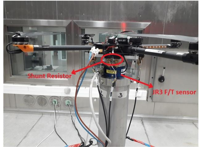
Fig. 3: Experimental setup for quad-rotor performance measurements.
