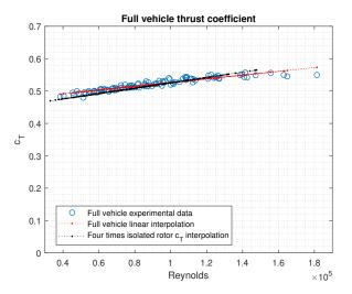
Fig. 16: Full vehicle thrust coefficient as a function of Reynolds number for all the environmental conditions.
