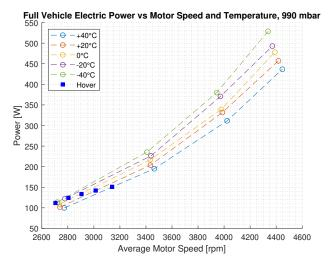
Fig. 15: Full vehicle electrical power as a function of motor speed for all the temperatures- 990 mbar.
