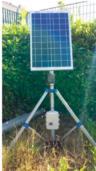
Figure 29. One of the nodes (enclosed in the white box) with its solar panel.
