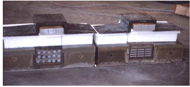
Fig. 3: Cross-section of the buried transmitter and the on board receiver of the PATH prototype [10].
