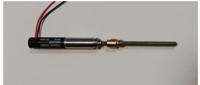
Fig. 3: The metal brush motor with the 4 stages gear reduction system and the preselected screw drive in the assembled configuration.
