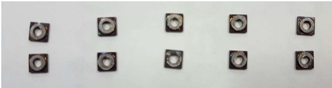
Figure 48: fracture surfaces after torsion test for THG5 samples (a); and TDHG samples (b)
