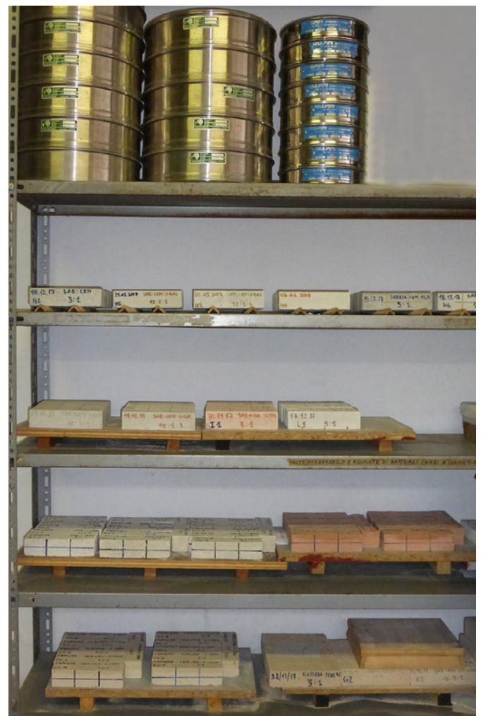
Fig. 6. DISEG Laboratory storage. Sets of mortar specimens of Group 1 (standard size, according to UNI EN 1015:2007).
