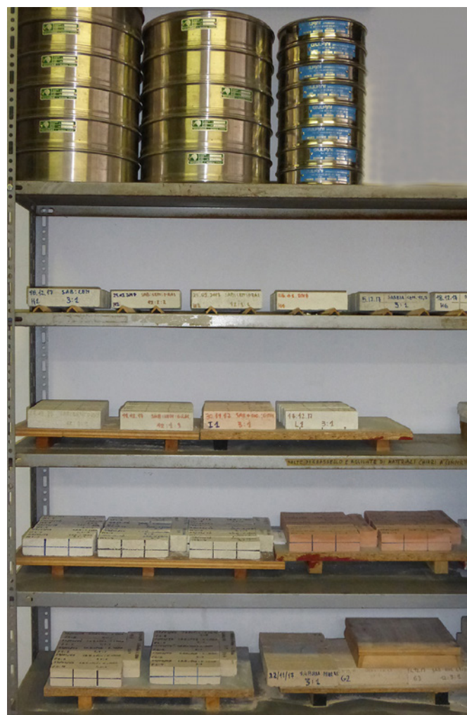
Fig. 6. DISEG Laboratory storage. Sets of mortar specimens of Group 1 (standard size, according to UNI EN 1015:2007).
