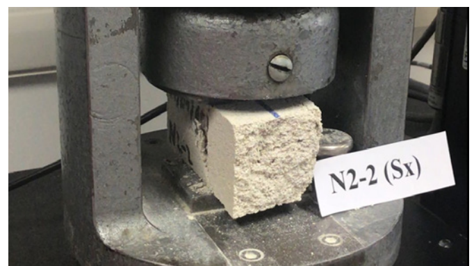
Fig. 7. Samples of set I, Group 1 tested to compression resistance according to UNI EN 1015-11:2007.
