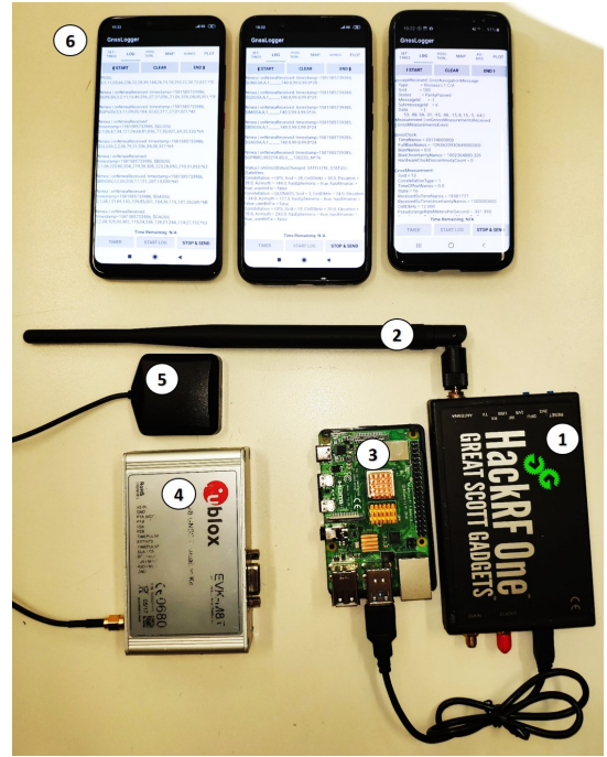
Fig. 2. Experimental setup consisting of a HackRF One, (1) equipped with an L1 stick antenna, (2), a Raspberry Pi 4B, (3) a u-blox™ Neo-M8N GNSS, (4) with an active GNSS antenna, (5) and a set of smartphones, (6) listed in Table I.
