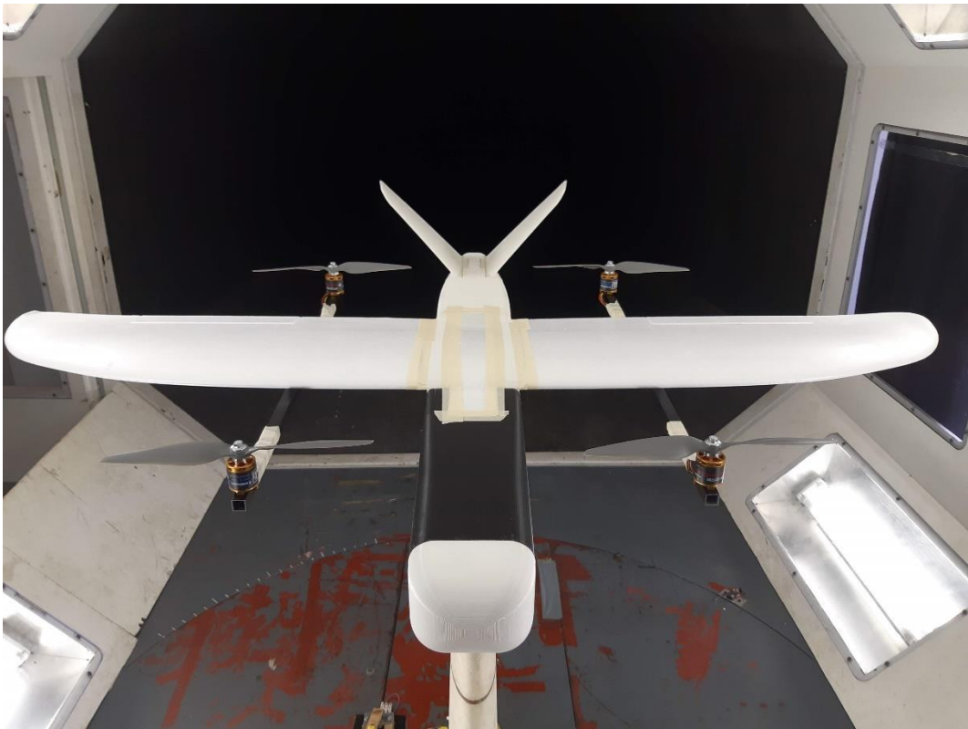
Figure 113: Mini Talon 3, propellers perpendicular to the airflow.
