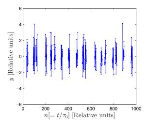
Fig. 15. Simulated frequency measurements for the sum of a WPM and a WFM with random blocks of missing data. The plot shows the first 1000 samples of a WPM+WFM noise. Within each of the 200 blocks made of 54 samples each, the position of the 15 WPM+WFM data is chosen randomly. This pattern of missing data is described in detail at the beginning of Sect. IV.R.
