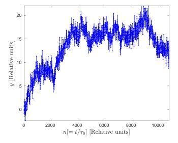
Fig. 19. Simulated frequency measurements for the sum of WFM and RWFM with blocks of missing data. This pattern of missing data is described in detail at the beginning of Sect. IV-B.
