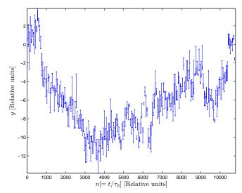
Fig. 21. Simulated frequency measurements for the sum of a WFM and an RWFM with blocks of missing data. This pattern of missing data is described in detail at the beginning of Sect. IV-B.
