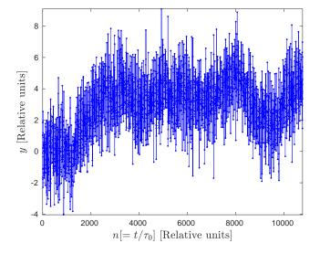
Fig. 17. Simulated frequency measurements for the sum of WPM and RWFM with blocks of missing data. This pattern of missing data is described in detail at the beginning of Sect. IV-B.
