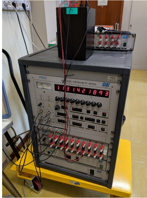
Figure 21 ASL F900 with the temperature-controlled reference resistance
