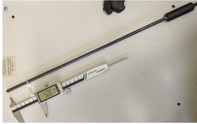
Figure 20 INRiM SPRT used in the experiment. The last 50 mm were inserted in the cavity metal block
