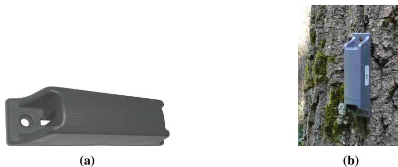
Figure 8. Sensor node package hosting the PCB, a half-AA battery and the normal mode helix antenna (NMHA) antenna. The aperture on the left improves the NTC thermal contact (a); fixed on trees with screws (b).
