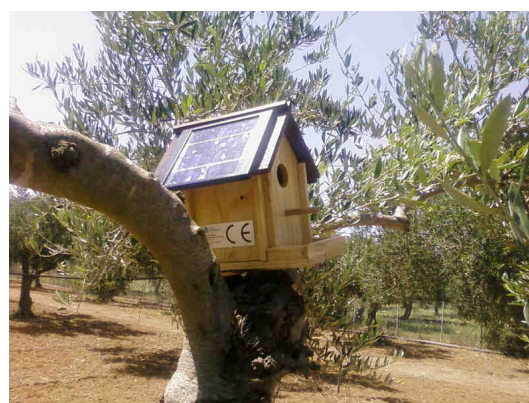
(b) Gateway 2 is deployed in the field high above the ground to improve its RF coverage. The ground of the test field is clean, facilitating navigation and sensor deployment and retrieval.
