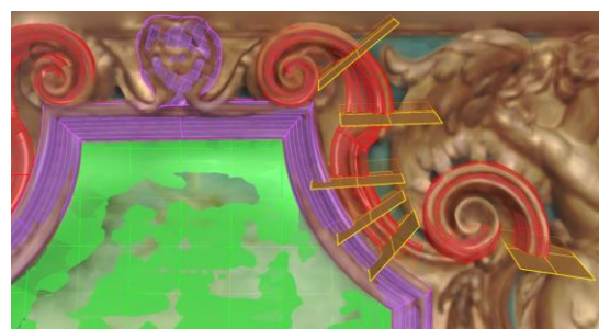
Figure 9. Example of reverse modelling starting from 3D mesh in Rhinoceros platform.
