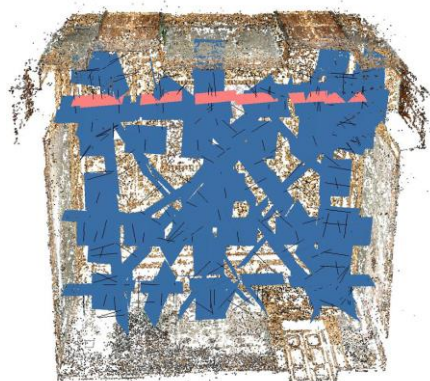
Figure 10. Co-registration between optical dataset (blue) and hyperspectral dataset (light orange).
