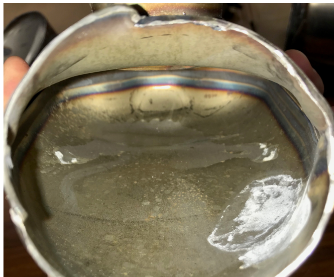
Figure 3.49: Urea deposits on System-B after the experimental campaign
