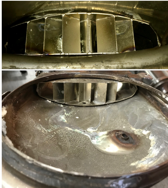
Figure 3.48: Urea deposits on System-A after the experimental campaign. Upper Mixer view (top) and bottom mixer view (bottom)
