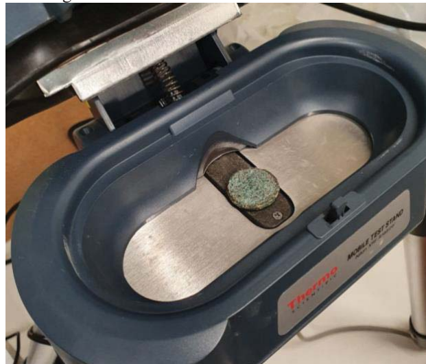
Fig. 3. Coin positioned for pXRF analysis.
