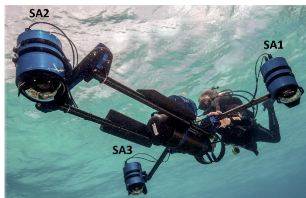
Figure 2. The SeaArray V4, a diver-operated tri-camera photogrammetry system employed in this research. In this article, the front camera is referred to as SA2, while the rear ones are respectively SA1 (left side) and SA3 (right side).
