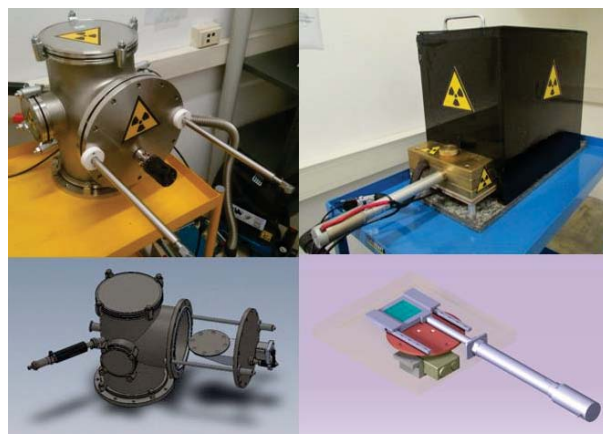
Fig. 1. On the left: \alpha irradiation system with the view of inner sample holder wheel. On the right: \beta irradiation system and its internal structure scheme.
