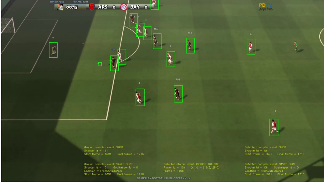
Figure 6: Example of scene generated by the Gameplay Football engine, with superimposed ground truth bounding boxes and IDs of each player and the ball. The ground truth and detected events are also overlaid on the bottom of the scene: in this frame, a shot attempt is correctly detected.
