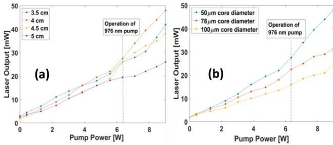
Fig. 3. (a) Average output power with different lengths of fiber #3. (b) Average output power of the amplified seed from EYPHFs #1-3 with length of 4 cm. The points represent actual measurements (connecting lines are just for clarity).
