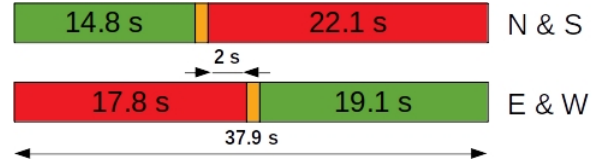
Fig. 4. Traffic light phases computed with Webster method.
