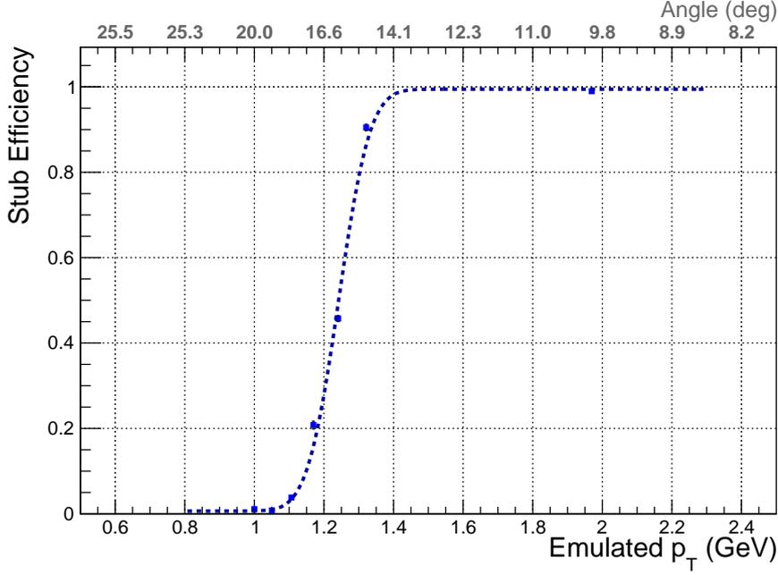
Figure 23: Stub efficiency of the full-size 2S module as a function of particle  $p_T$  measured at the Fermilab beam test facility during the angular scan. The module was operated at a bias voltage of 250 V and the  $V_{CTH}$  value was set to 92. A radius of 60 cm is used to convert the beam incident angle to effective  $p_T$ .
