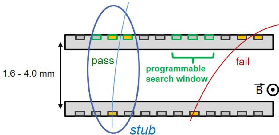
Figure 2: Illustration of the  $p_T$  module concept [3]. Correlation of signals in closely spaced sensors enables rejection of low- $p_T$  particles. The channels shown in green represent the selection window to define an accepted stub; a low- $p_T$  rejected track is shown in red.
