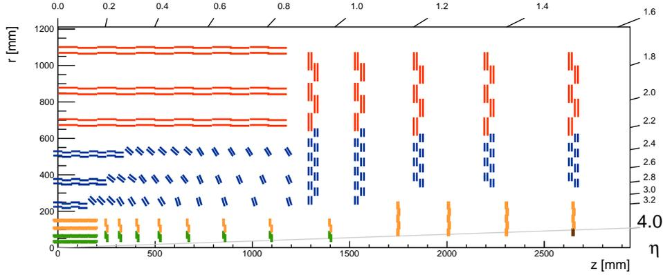
Figure 1: Sketch of one quarter of the tracker layout in  $r - z$  view. The radial region below 200 mm is referred to as Inner Tracker and will be instrumented with pixel modules. In the Outer Tracker, the radial region between 200 and 600 mm is equipped with PS modules (blue lines), while the region beyond 600 mm will be populated with 2S modules (red lines). The CMS coordinate system is defined in Ref. [1].
