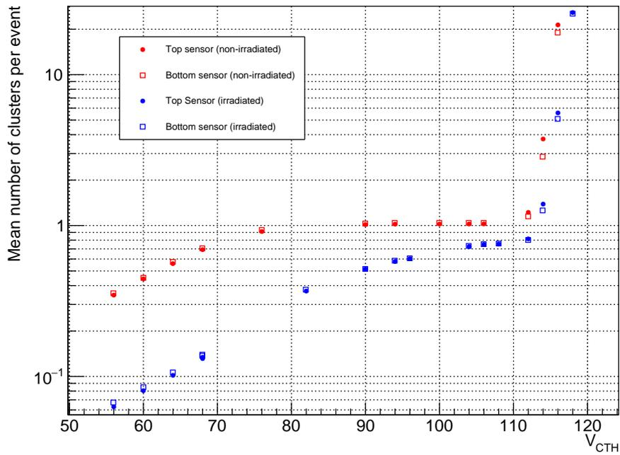
Figure 14: Average number of clusters per event for non-irradiated and irradiated sensors as a function of  $V_{CTH}$ . A bias voltage of 250 V (600 V) was applied to the non-irradiated (irradiated) mini-module.
