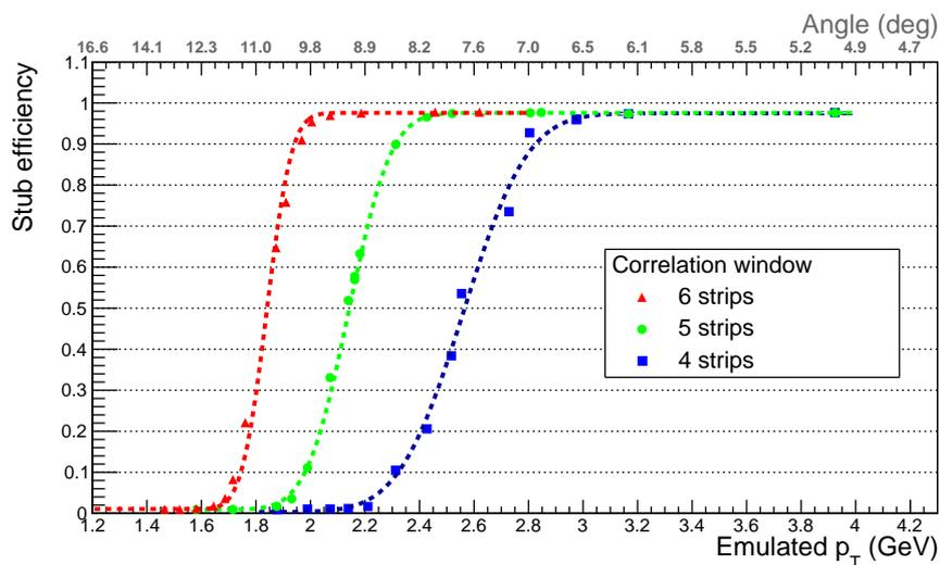
Figure 21: Stub efficiency comparison of different angular scans with different correlation windows for the irradiated module. The choice of window size leads to a shift in the turn-on  $p_T$ , but the efficiency at the plateau remains the same. A bias voltage of 600 V was applied to the irradiated mini-module.
