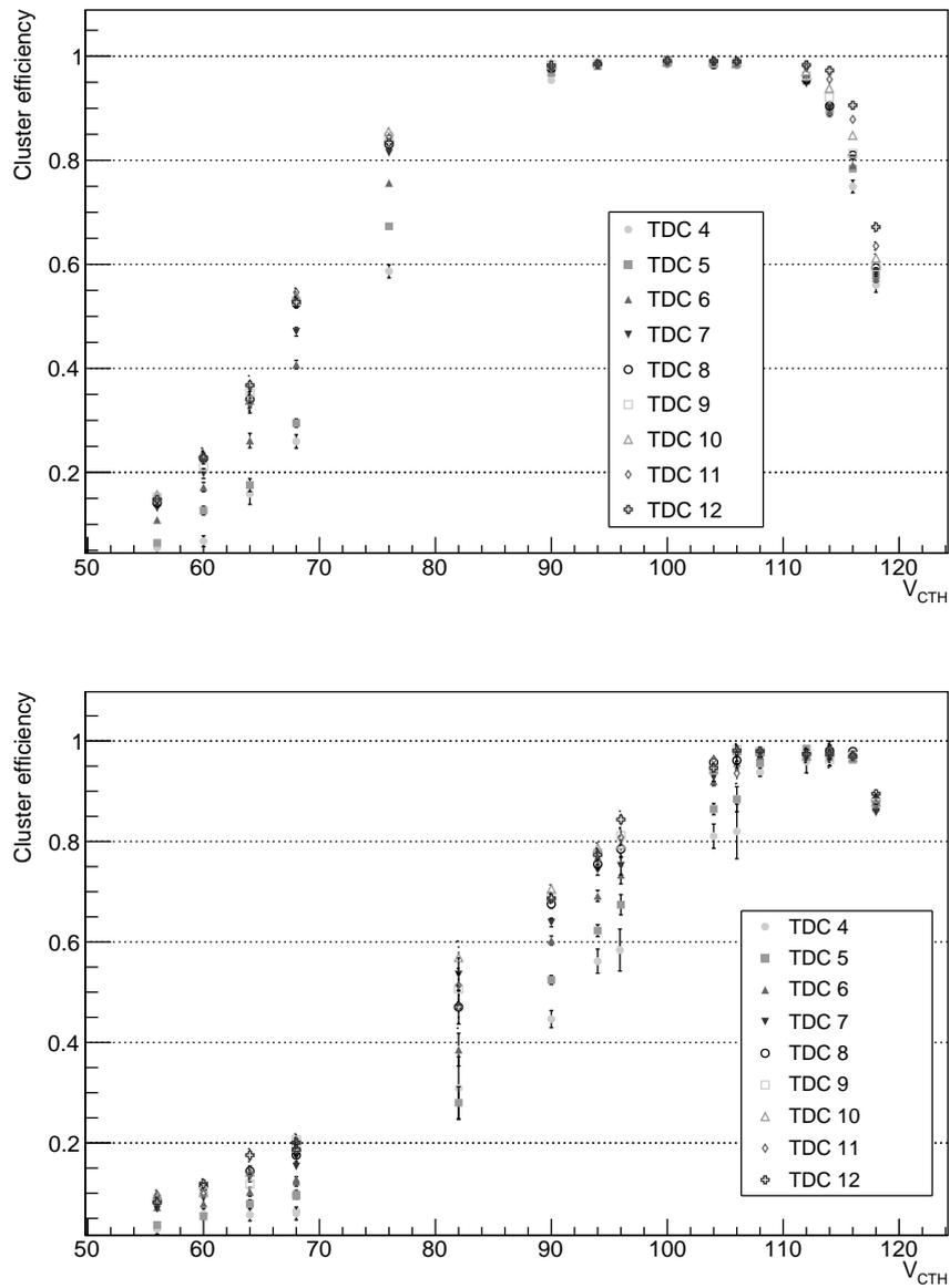
Figure 16: Cluster efficiency of the non-irradiated (top) and irradiated (bottom) 2S mini-modules presented as a function of  $V_{CTH}$  for different phase differences between trigger and readout clocks. A bias voltage of 250 V (600 V) was applied to the non-irradiated (irradiated) mini-module.
