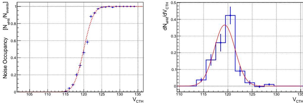
Figure 9: S-curve measured for a single input channel on one of the two CBC2s on a non-irradiated prototype module at room temperature with the sensor biased at 250 V. On the left the measured data are shown along with a fit to the measured data performed using Eq. 1, while on the right the differential histogram is shown with the corresponding Gaussian fit.
