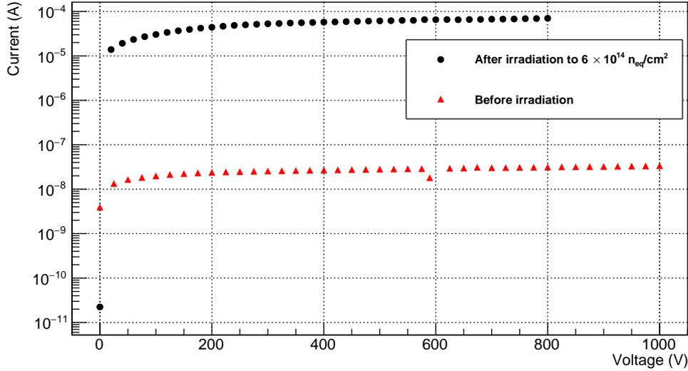
Figure 6: The current-voltage characteristic of a sensor of the mini-module before (red) and after (black) irradiation to  $6 \times 10^{14} \text{ n}_{\text{eq}}/\text{cm}^2$ , showing the increased current after irradiation. The measurements were taken at  $-20^\circ \text{C}$  and  $20^\circ \text{C}$  for the irradiated and non-irradiated sensors, respectively.
