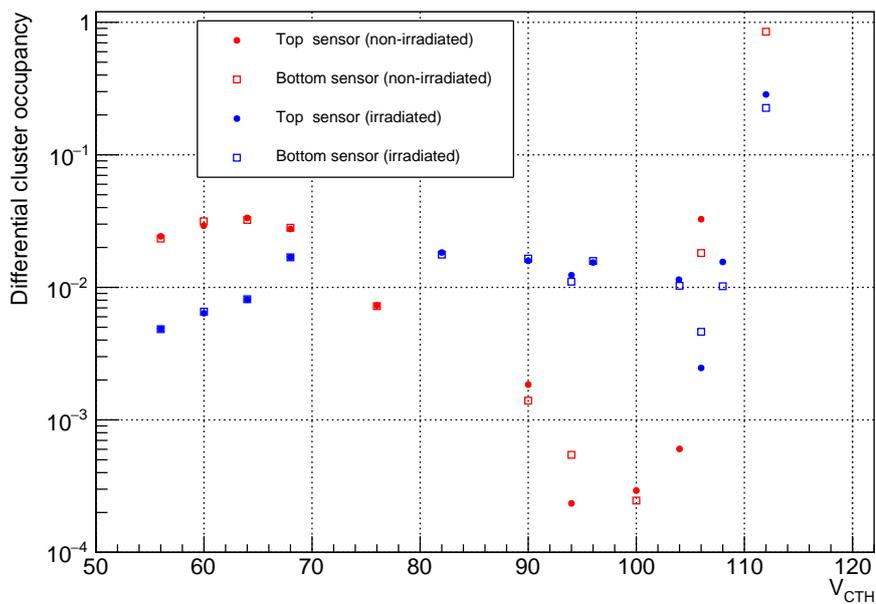
Figure 15: Differential cluster occupancy for non-irradiated and irradiated sensors as a function of  $V_{CTH}$ . A bias voltage of 250 V (600 V) was applied to the non-irradiated (irradiated) mini-module.
