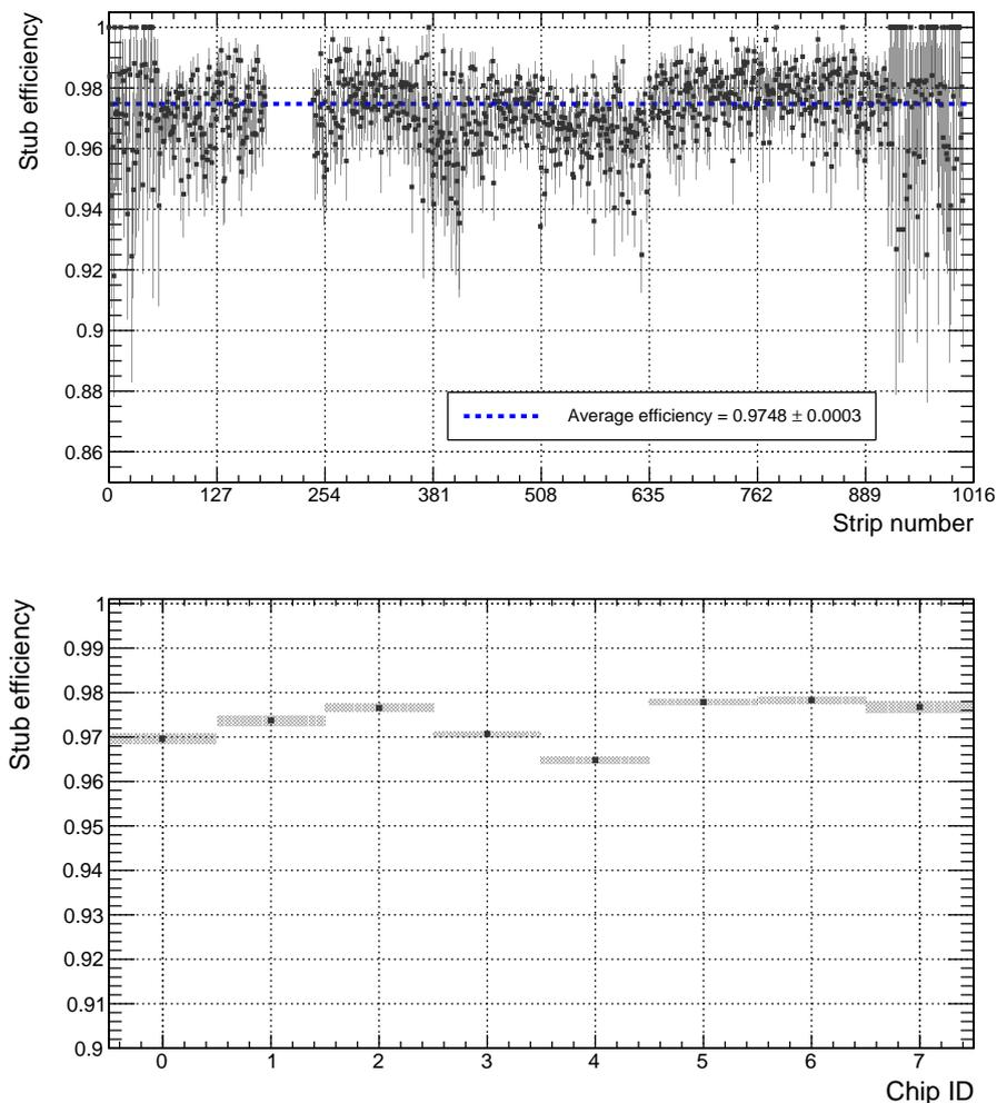
Figure 22: Stub efficiency of a full-size 2S module measured at the CERN beam test facility. The module was operated at a bias voltage of 250V and the  $V_{CTH}$  value was set to 115 DAC units. Top: stub efficiency per strip, bottom: stub efficiency per chip computed using data from strips scanned by the beam.
