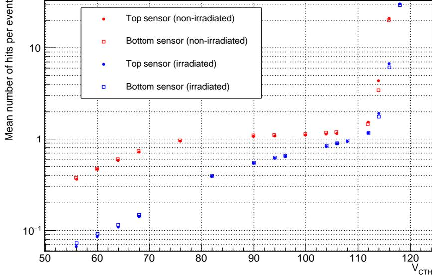
Figure 13: Average number of hits per event on non-irradiated and irradiated sensors as a function of  $V_{CTH}$ . A bias voltage of 250 V (600 V) was applied to the non-irradiated (irradiated) mini-module.
